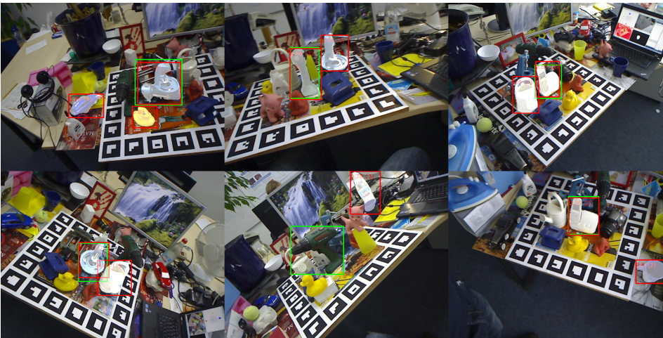
Figure 7.3: The trained Mask R-CNN [13] network evaluated on LineMOD [14], including predicted segmentation masks and labels
