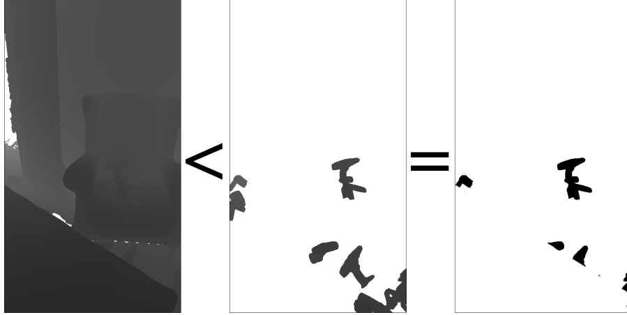
Figure 6.3: A blended depth map, an object depth map and the resulting occlusion mask
