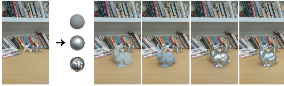
Figure 3.11: The LDR input, its inferred lighting and a comparison of each a real and rendered object with matte and reflective materials [20]
