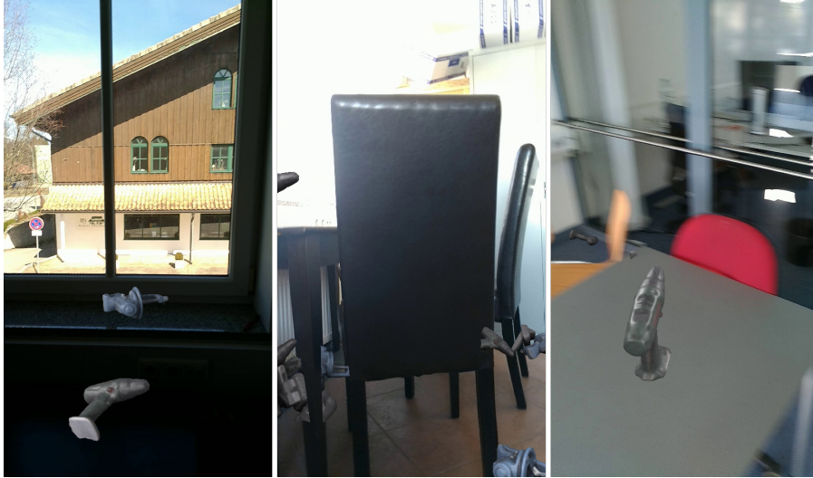
Figure 8.1: Lighting not matching scene illumination, "clipping" due to an inaccurate scene mesh, low quality result due to undetected blur (left to right)
