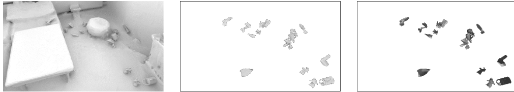
Figure 6.5: Ambient occlusion of objects and scene, objects rendered without scene influence, objects rendered with the scene included for indirect illumination (left to right)
